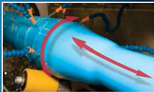
Stretching regular PVC pipe biaxially in both the hoop and axial directions — lengthways and sideways — over a mandrel after the pipe is extruded dramatically improves the performance of PVC material.
